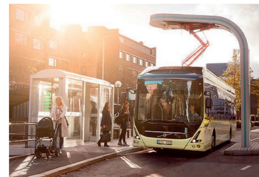
Figure 3.1.7. Fast charging station at the end of bus line
