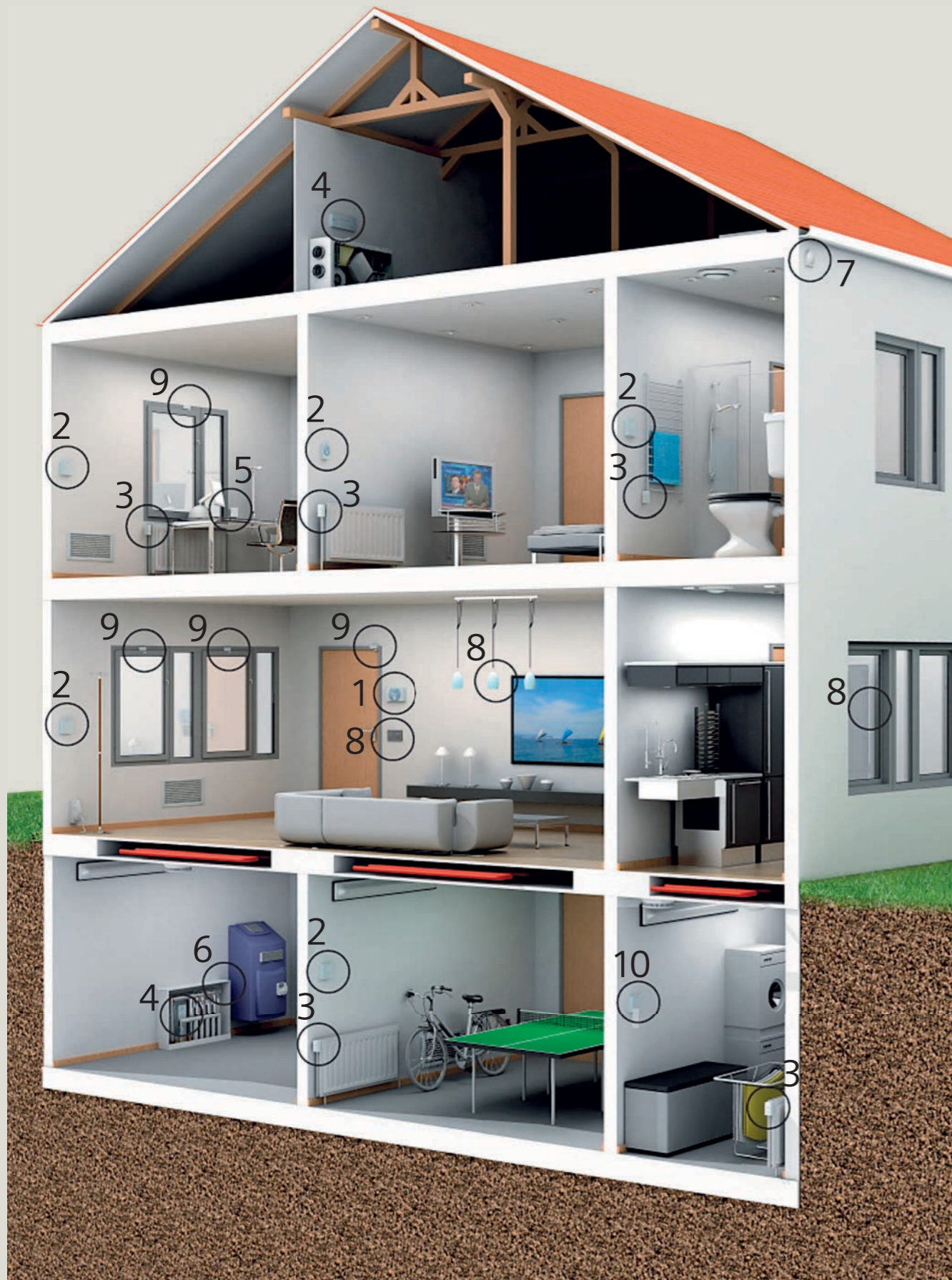
Figure 2.1.16 BMS for a single building [Siemens]
