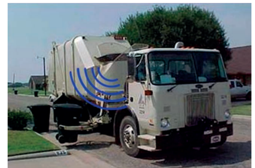
Figure 3.2.4. Reading RFID label of container
