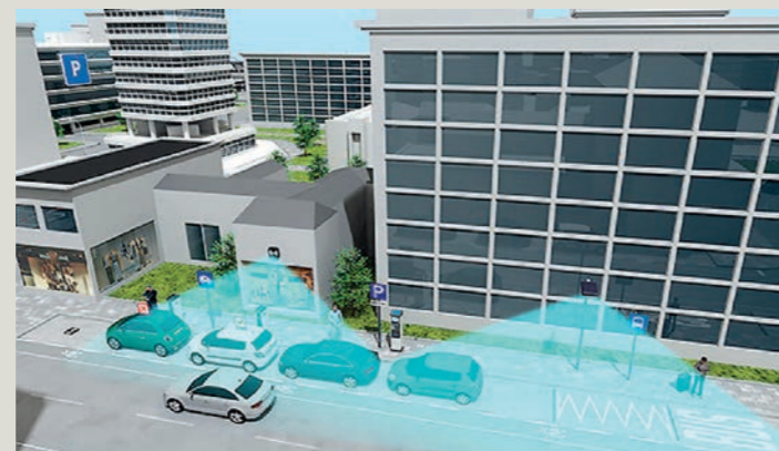
Figure 3.2.7. Example of sensors located on existing objects
