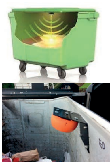
Figure 3.2.2. Examples of sensors in waste containers
